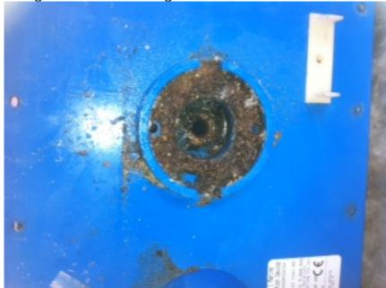
**Electrical fault** - The ElectraSan is normally installed in a moist environment and hence its electrical components are exposed to corrosion risk. The blue plastic cover does protect the electrical components but not adequate enough to safely shield them.
